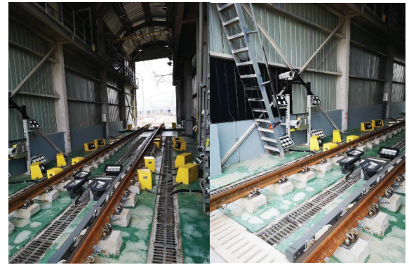
Fig. 1. The actual scene of the TEDS. When the EMUs enters the station at a constant speed, the line scan camera deployed at the throat will collect the image information of the EMUs and determine its health status.
